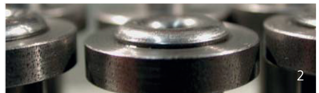
Rivet with nominal size – result: good
