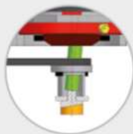
Touch probe on work piece and forming begins
