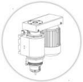
Unit with lateral mounted motor
