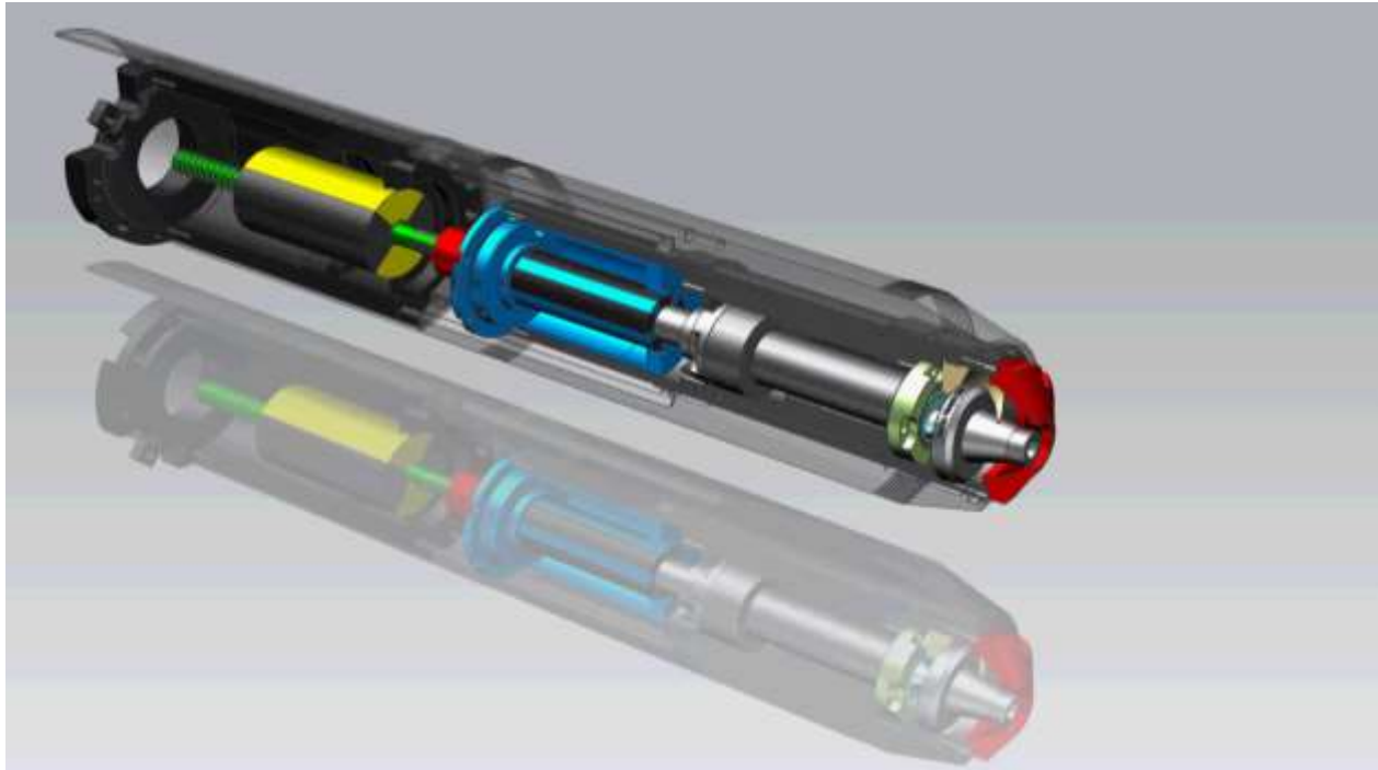
Principle concept of ELECTRIC – inline servo driven
